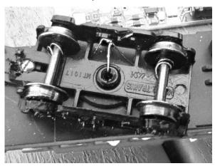
Be sure to pre-tin the magnet wire. Sustained heat is needed for the hot solder to burn off the insulation on the magnet wire. Then bend a hook in the wire to secure the wires to each other and solder them.
