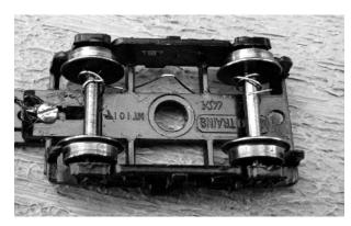
Insert and bend the phosphor bronze wire as shown above. Keep the loops on the end loose to minimize drag. The phosphor bronze wire should be next to the non-insulated side of the wheels (no insulation between the wheel and the axle).
