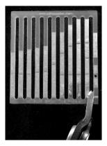
2. Free throw bar by cutting the the sprue parallel to the length of the tie.
